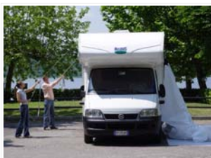
Streight forward set up system. Using 2 ropes you can pull the cover on the roof without using the ladders.
